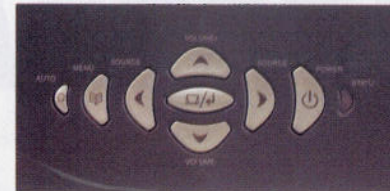
The top panel offers control for menu, source, keystone, volume and power.
