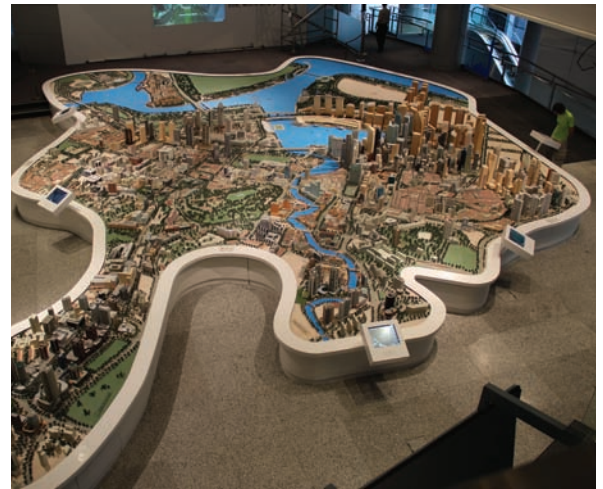
Above: 4 Titan Projectors utilising the built in Warp and Blend functionality to accurately project onto an expansive 3D model of Singapore
